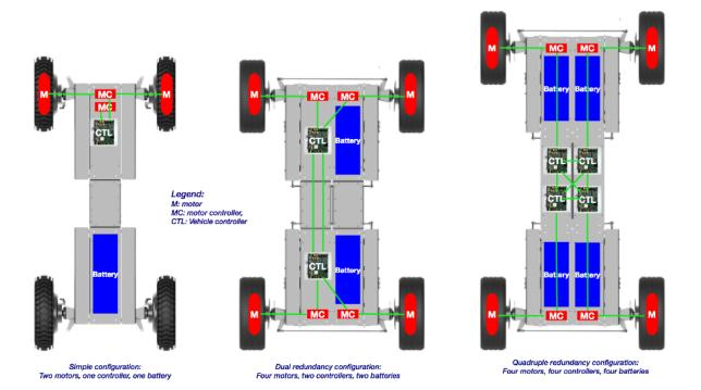
For vehicles require more safety and security we apply our own ARRL (Assured Reliability and Resilience) criterion. This criterion defines architectures that take into account the fault behavior and its consequences on the continued operation of a mission or safety critical system.
