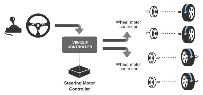
All of the sections are galvanically isolated to reduce common mode failures but communicate using high speed interconnects (typically ethernet or optical fiber) configured in a redundant mesh. This provides the advantages of reduced wiring, a principle that is also applied to peripheral nodes like sensors and actuators.
